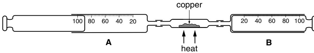
Syringe **A** contained 90 cm<sup>3</sup> of air. The air was forced over heated copper into syringe **B**. The air was then forced back into syringe **A**.
